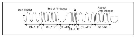
Figure 2-6. Continuous Trigger Mode
